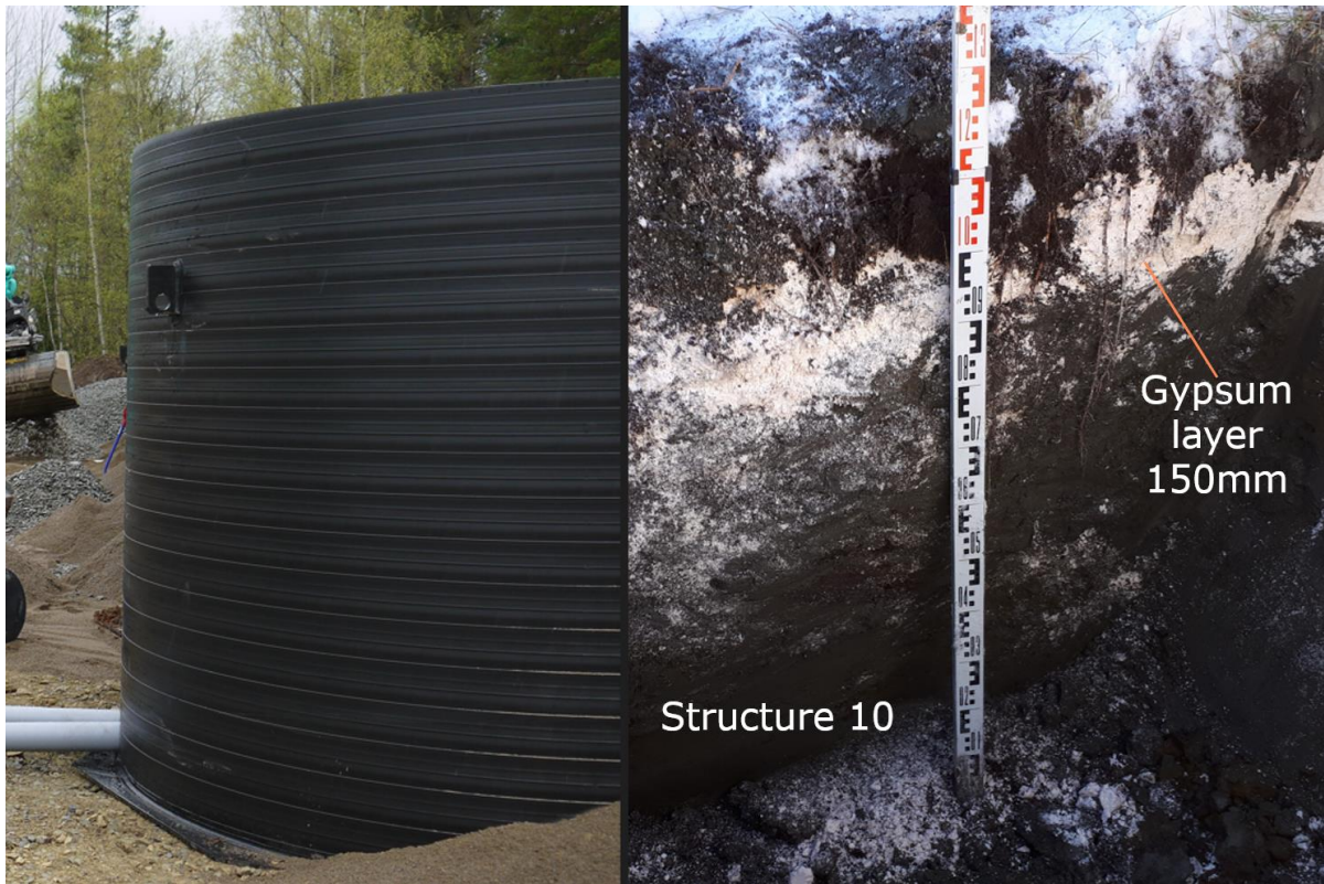
Figure 3. Test tank on left and layer structure on right from disassembly phase.
